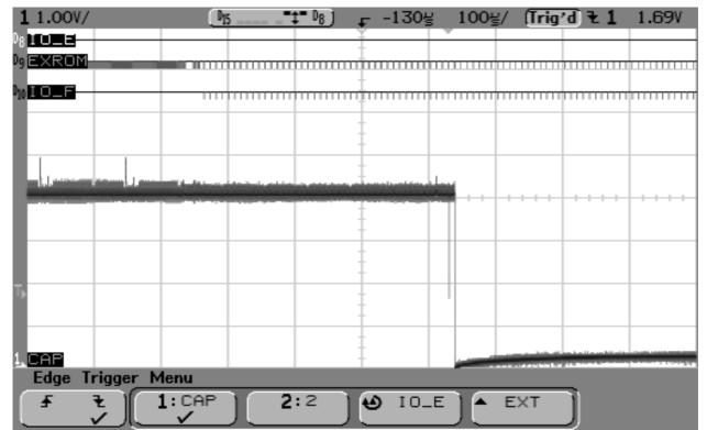
The analog channel in this diagram is on pin 6 (nQ output of the RS flipflop). Funny: Exactly 42 accesses are necessary to make the flipflop switch. Now we have the question to the answer that Deep Thought gave us :-) Note that this is a statistical process. It will take more accesses with a badline, and it'll take more accesses on a new board, as IO accesses are about 50-100ns shorter.
