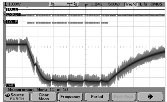
When switching on, the computer turns off the \$8000 rom. The capacitor voltage drops while addresses in \$dfxx are accessed, and it rises when these registers are left alone. Note that a badline interrupts the loop, as this enlarged diagram shows:
